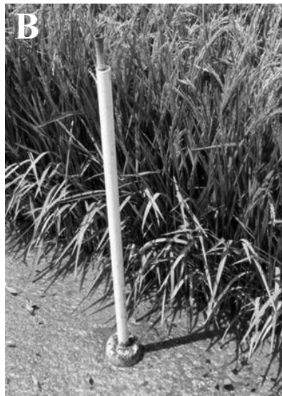
Figure 6. Overhead sprinkler irrigation of rice in Arkansas (A). Simple depth gauge consisting of seine float attached to PVC pipe being used to help manage rice flood (B). (Sprinkler rice photo credit: Dr. Brian Ottis, RiceTec.)
